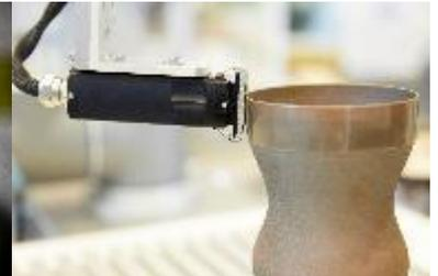
*Non-destructive testing of parts made using additive manufacturing techniques. ©CEA*
