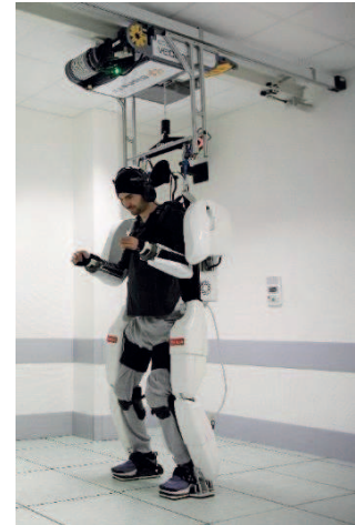
The four-limb exoskeleton controlled by the patient during the BCI project at Clineatoc ©Clineatoc
